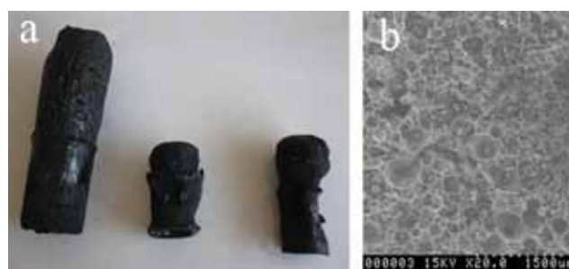
Figure 2 (a) Photograph of glutaraldehyde foam and glyoxal foams; (b) SEM image of a typical glutaraldehyde foam.
