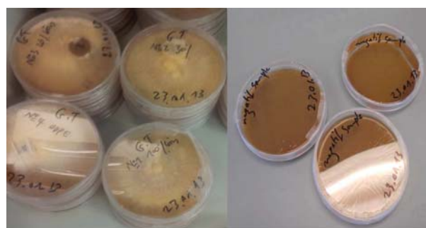
Figure 2 Composite samples exposed to microbial attack (left) and negative samples (right).
