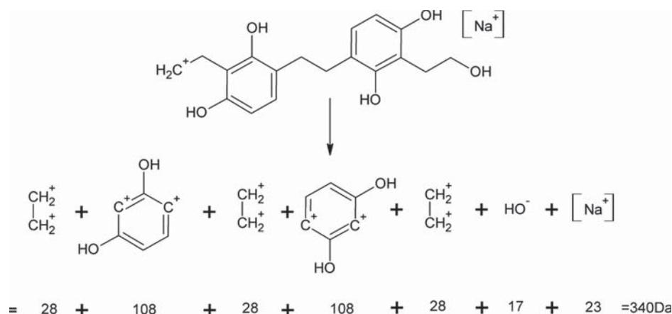
**Figure 1** Example of combination for the 340Da peak.
