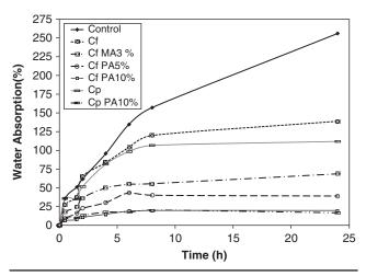
**Figure 5** Water absorption of soy plastics resin formulations with cotton fiber and cotton powder over 24 h of exposure to water steeping.
