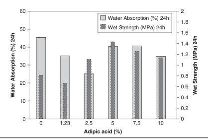
Figure 8 Water absorption and wet strength of adipic acid based soy plastics resin formulations with PA5% as the base material.
