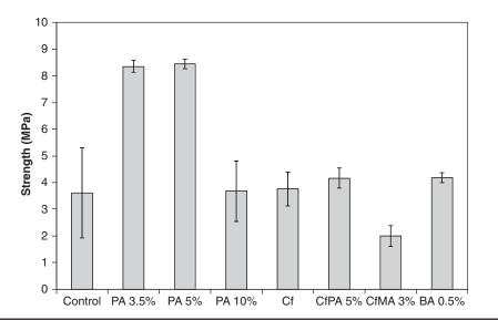
Figure 1 Dry state strength of phthalic anhydride and composite soy plastic resin formulations.
