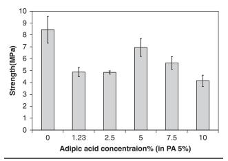
**Figure 7** Dry state strength of adipic acid based soy plastics resin formulations with PA5% as the base material.
