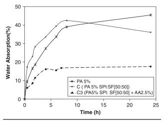
**Figure 11** Water absorption of PA 5% formulation compared with corresponding 50:50- SPI : SF based plastic formulations over 24 h of exposure to water.
