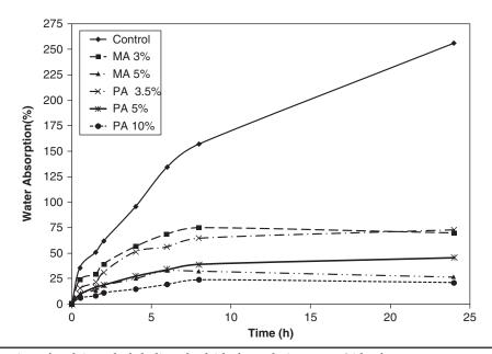
Figure 2 Water absorption of maleic and phthalic anhydride formulations over 24 h of exposure to water.
