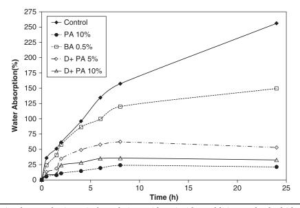
Figure 3 Water absorption for soy plastics resin formulations with antioxidant additives and anhydride with salts over 24 h.
