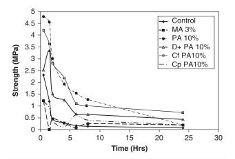
Figure 6 Wet state tensile strength at intermittent intervals over 24 h of exposure to water.
