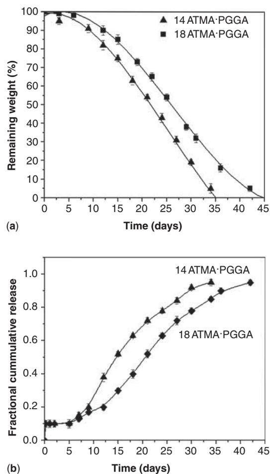
**Figure 18** a) Hydrolytic degradation profiles of  $n$ ATMA-PGGA complexes incubated at pH 7.4 and 37°C, and b) cumulative releasing profile of erythromycin from complexes loaded with 10% of drug. (From reference [67] with permission).
