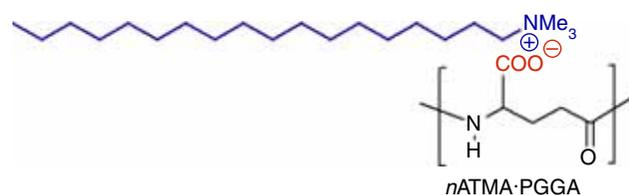
**Figure 16** Stoichiometric complexes of PGGA with alkyltrimethylammonium surfactants.
