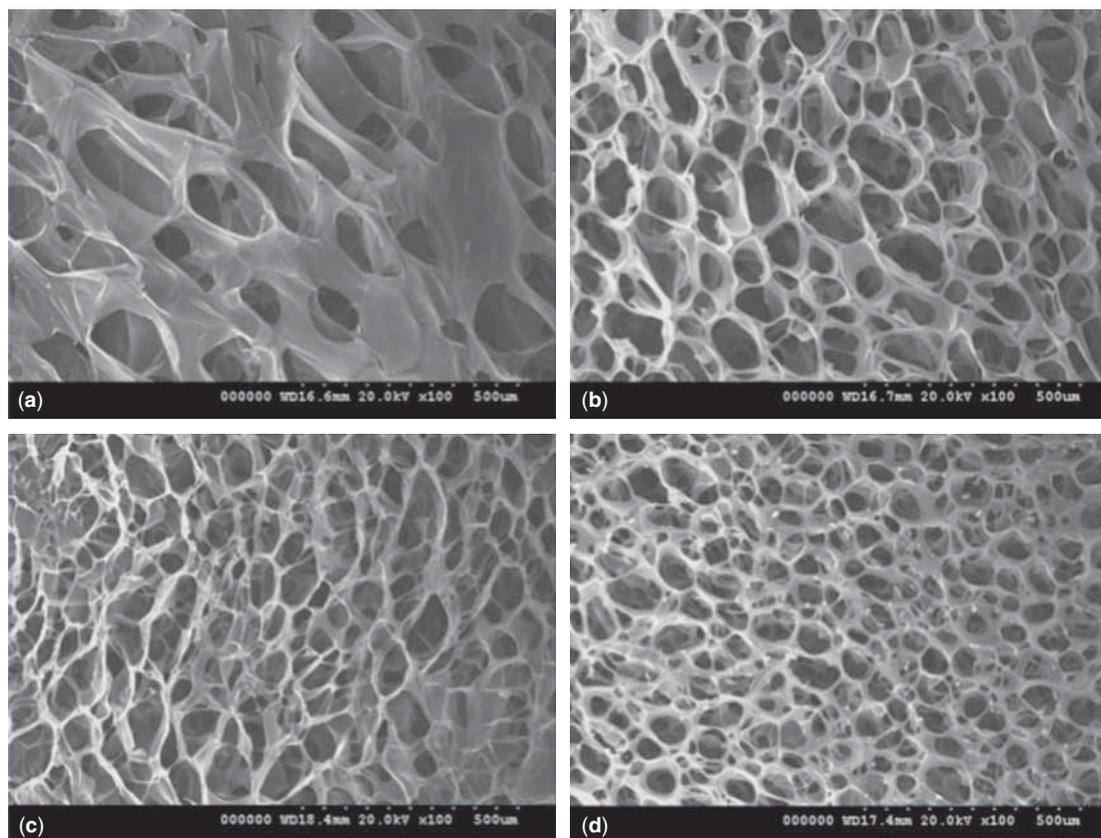
**Figure 19** SEM micrographs of the surface of the hydrogel made of CS-PGGA complex for different PGGA/CS ratios (w/w): a) 0.1, b) 0.2, (c) 0.6, and (d) 1.0. (From reference [68] with permission).
