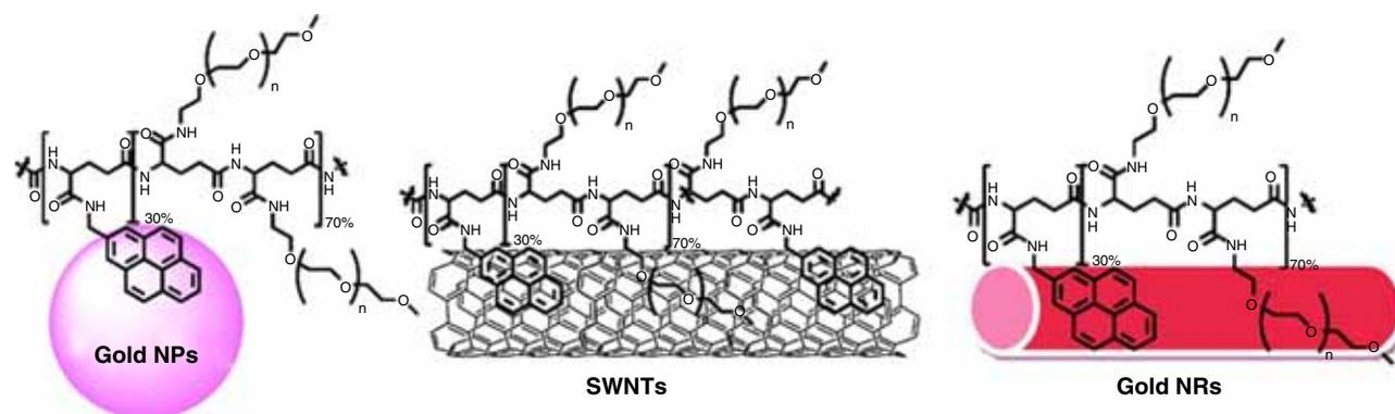
**Figure 14** Gold nanoparticles, single-wall nanotubes and gold nanorods coated with PEG-graft-PGGA functionalized with pyrene. (From reference [58] with permission).
