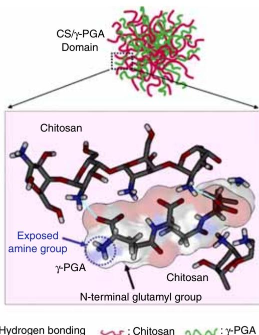
**Figure 22** Structure of the CS- $\gamma$ -PGA complex resulting from molecular dynamic simulations showing intermolecular hydrogen bonding and the exposed *N*-terminal amine group in  $\gamma$ -PGA. (From reference [72] with permission).
