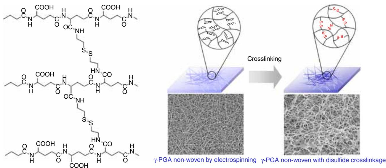
**Figure 13** a) Network of PGGA crosslinked with cystamine. b) Schematic illustration of the fabrication of PGGA nonwovens and cell proliferation on the substrate. (From reference [50] with permission).
