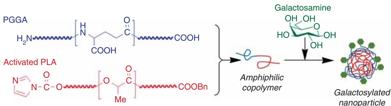
**Figure 15** Synthesis of PLA-block-PGGA copolymer and structure of their shell-core nanoparticles functionalized with L-galactosamine. (Adapted from reference [61] with permission).
