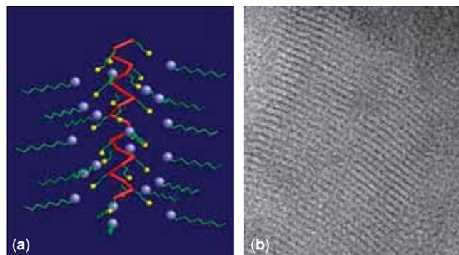
**Figure 17** a) The molecular structure of  $n$ ATMA-PGGA complexes. b) TEM micrograph of the 22ATMA-PGGA complex. (From reference [66] with permission).
