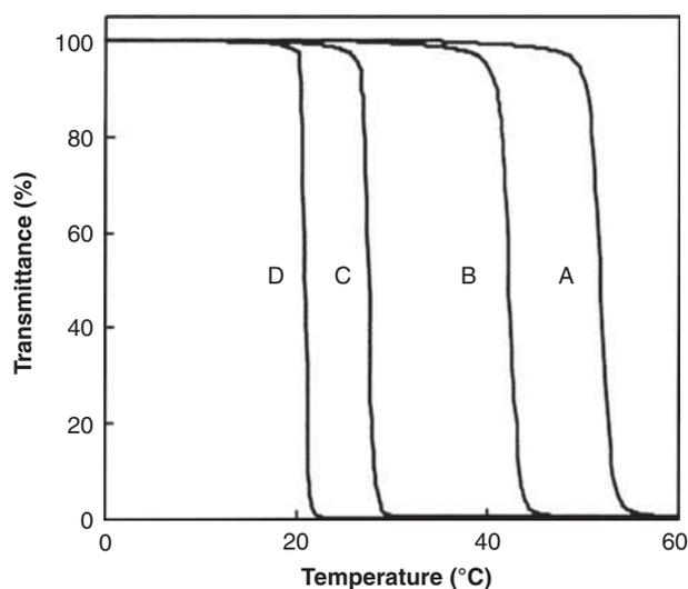
**Figure 12** Effect of temperature on turbidity of 1 wt % aqueous solution of PGGA amidated with mixtures of aminoalkanoles at different ratios and compositions (A to D) (see reference for meaning of labels). (From reference [43] with permission).
