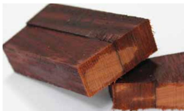
Figure 3 Photograph of sections of Paduk welded wood joints after immersion in water for 20 days showing the lighter wood colour zone surrounding the weld line indicating that no water has reached it.
