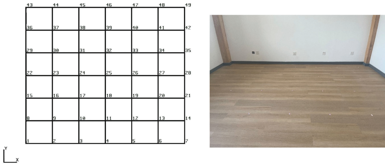
(a) Meshing diagram of the modal model of the floor structure of Room A
