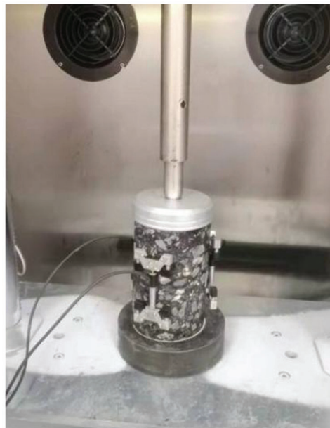
Figure 3: Dynamic modulus test
