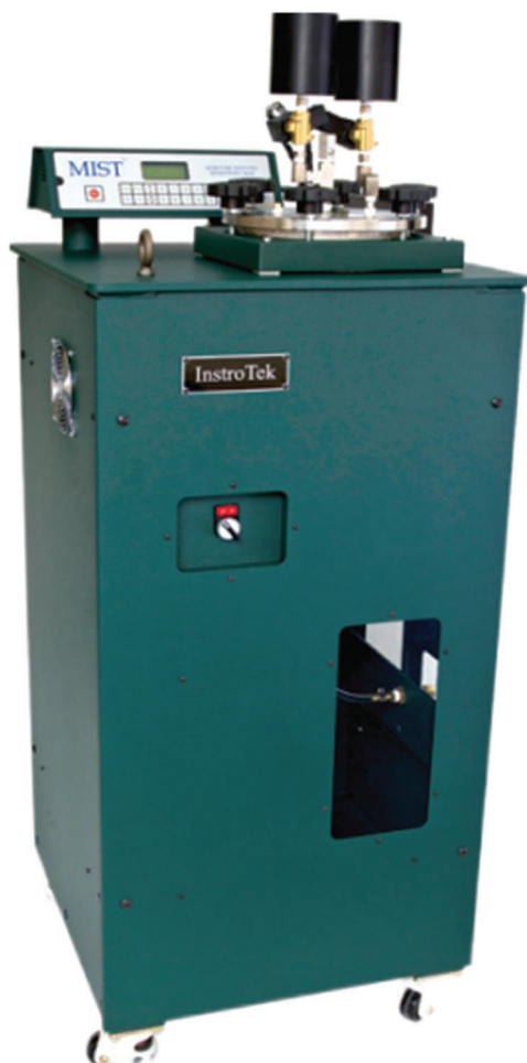
Figure 2: Moisture induced stress tester (MIST)
