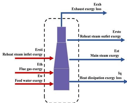
**Fig. 2** Calculation exergy efficiency range of primary intermediate reheat boiler
