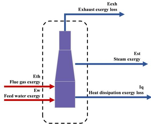
**Fig. 1** Calculation range of Exergy efficiency of CDQ waste heat boiler
