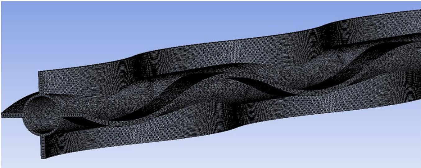
Fig. 2: Meshed model of the wavy fin turbulator (CR =2)
