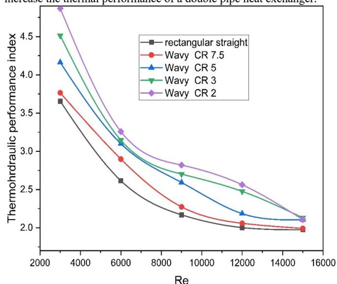
**Fig. 16:** Variation of THPI with Re for various turbulator configurations
