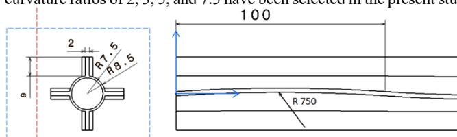
**Fig. 1:** Geometrical specifications of the wavy turbulator.
