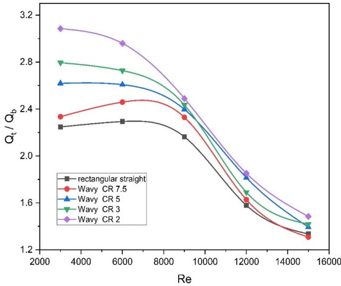
**Fig. 13:** Variation of  $Q_t/Q_b$  with Re for various turbulator configurations
