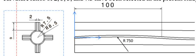
**Fig. 1:** Geometrical specifications of the wavy turbulator.
