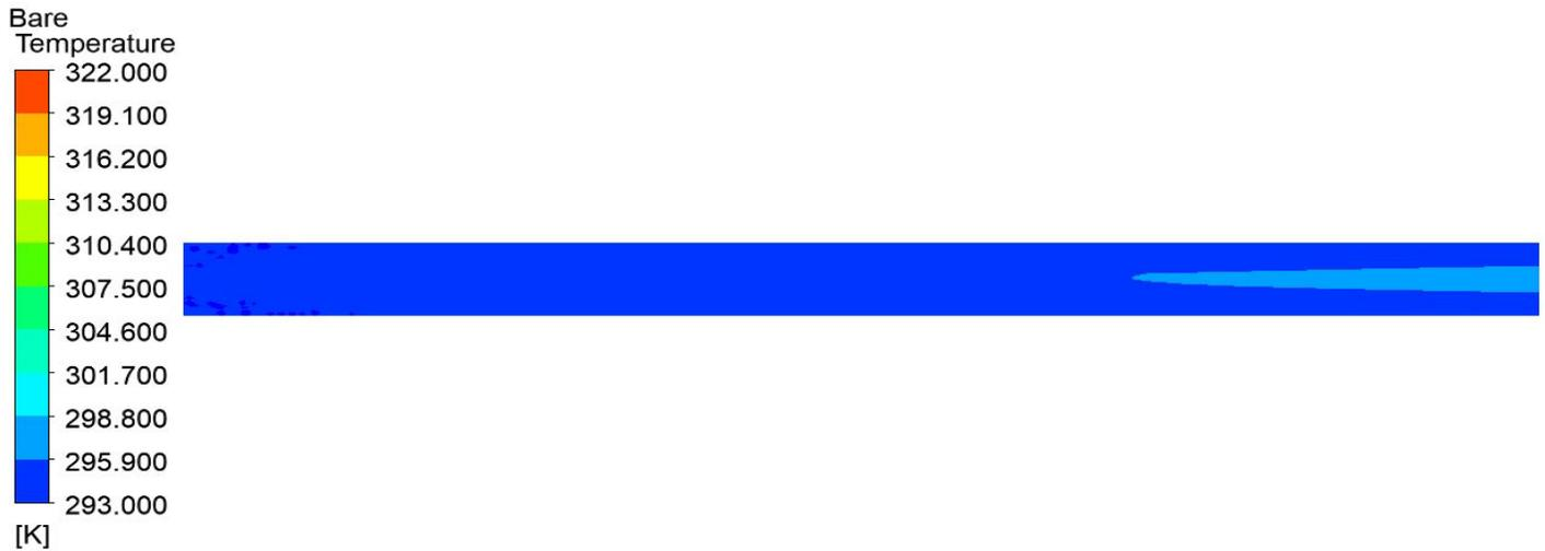
Fig. 7: Temperature distribution of air along the length for the bare pipe
