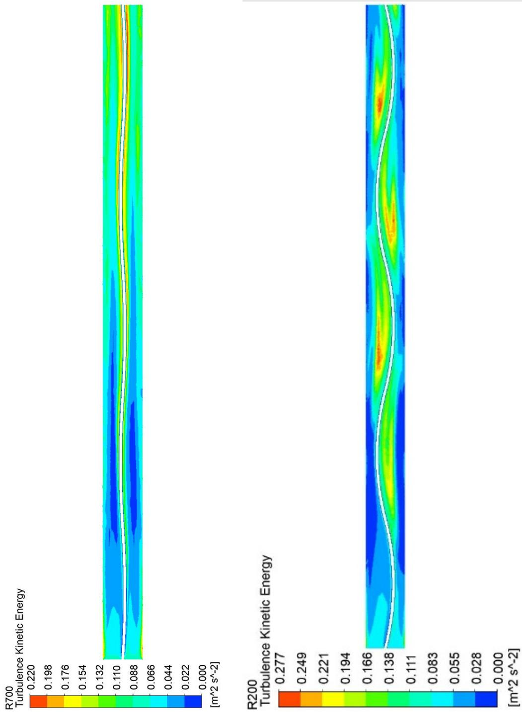
**Fig. 10:** Distribution of turbulent kinetic energy of air along the length for the wavy tubulator for CR =7 and CR =2
