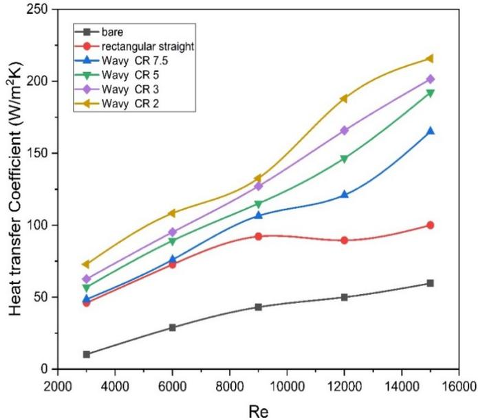
**Fig. 14:** Variation of convective Heat transfer coefficient with Re for various turbulator configurations
