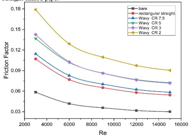
**Fig. 15:** Variation of friction factor  $f$  with Re for various turbulator configurations
