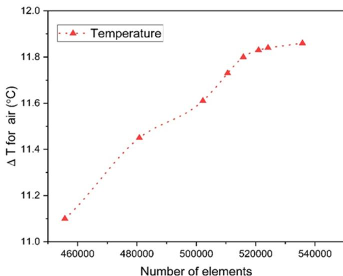
**Fig. 3:** Grid independence test for the wavy fin turbulator (CR =2, Re=6000)
