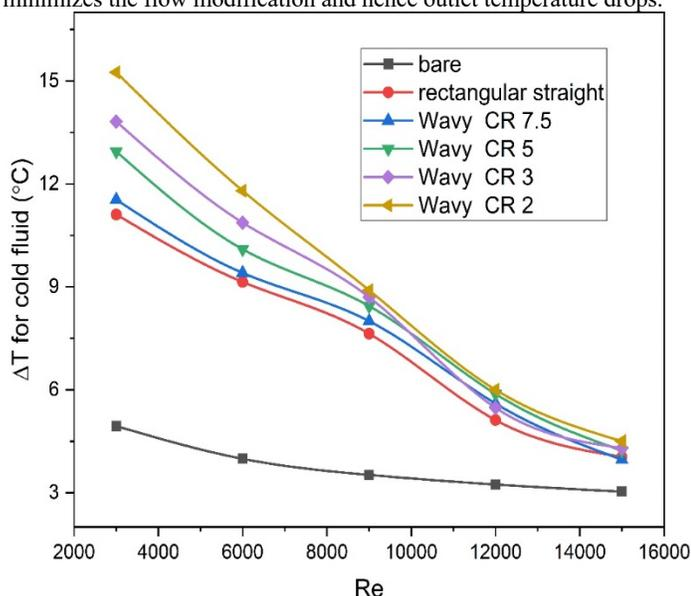
Fig. 11: Variation of  $\Delta T$  for the air with Re for various turbulator configurations
