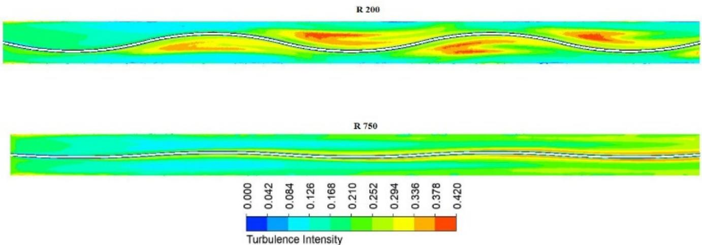
Fig. 9: Distribution of turbulent intensity of air along the length for the wavy turbulator for CR =7.5 and CR =2
