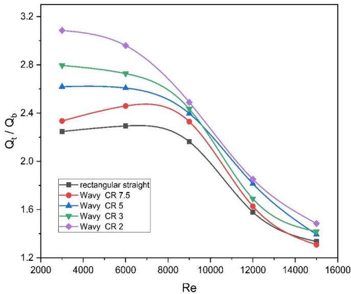
**Fig. 13:** Variation of  $Q_t/Q_b$  with Re for various turbulator configurations
