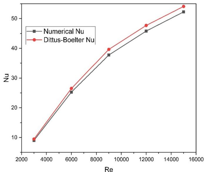
**Fig. 4:** Comparison between the CFD predicted and analytical values for  $Nu$
