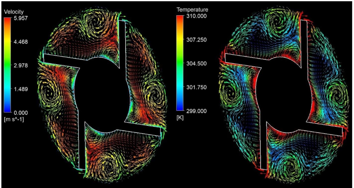
Fig. 5: Velocity and temperature contour for the air domain in a vertical plane for the wavy fin turbulator (CR=2)
