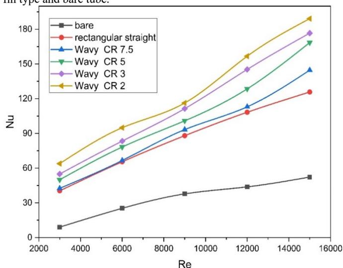
Fig. 12: Variation of Nu with Re for various turbulator configurations
