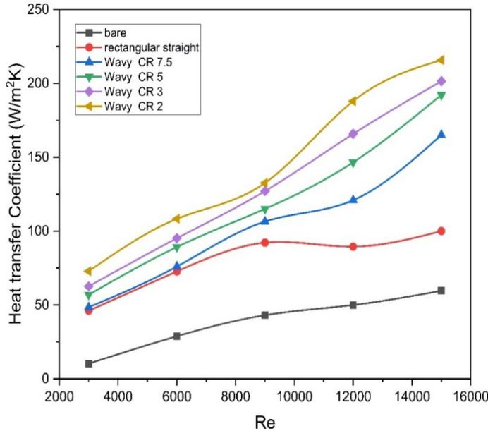
**Fig. 14:** Variation of convective Heat transfer coefficient with Re for various turbulator configurations
