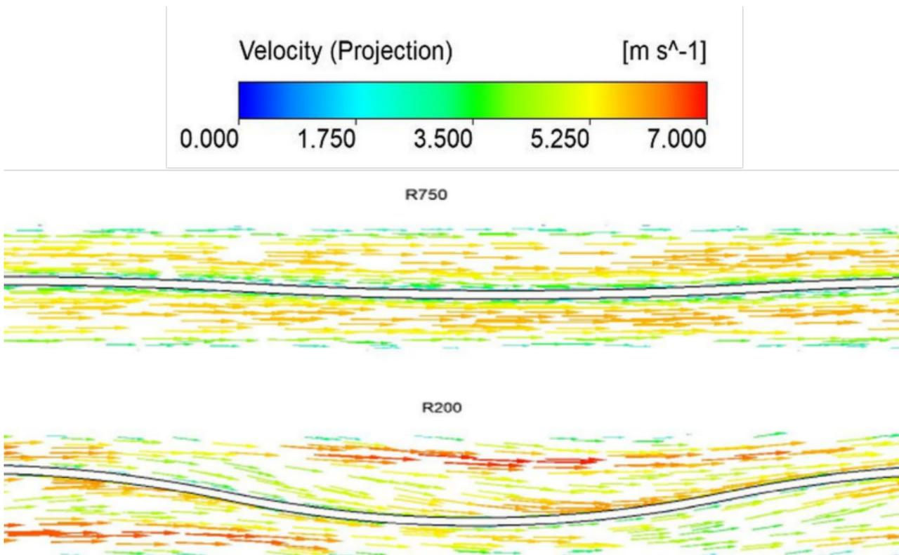
Fig. 6: Velocity plots for wavy fin turbulators in an isoplane coloured with velocity values
