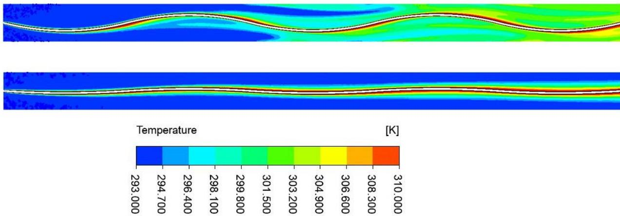
Fig. 8: Temperature distribution of air along the length for the wavy turbulator for CR =2 and CR =7.5
