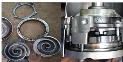
**Fig.9** Stationary & Rotating Scrolls, Oldham coupling, and assembled scroll-type expander
