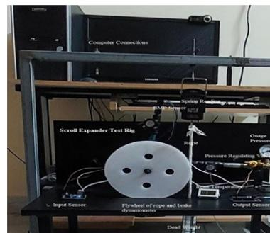
**Fig. 11** Scroll expander test setup
