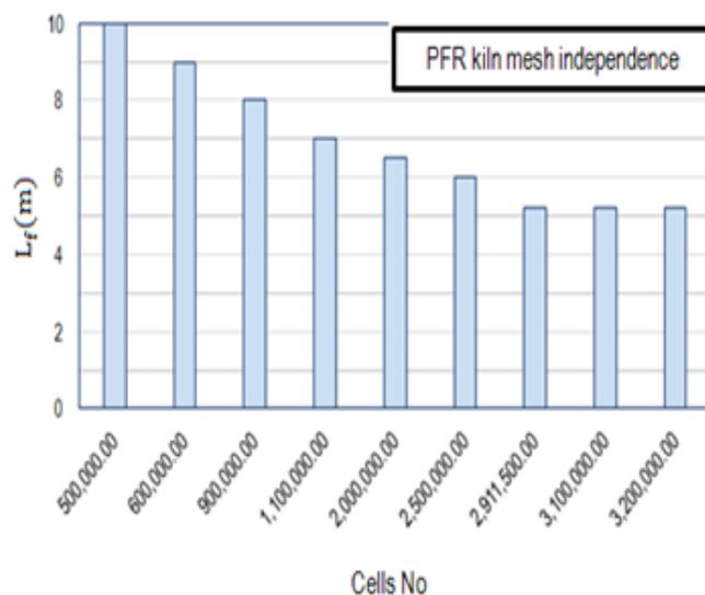
Fig. 2 Grid generation and grid independence study for PFR shaft kilns
