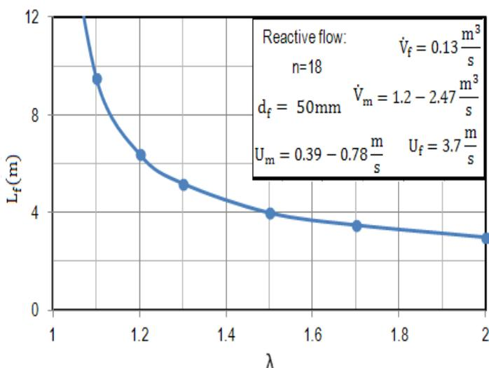
Fig. 8 Influence of excess air number on flame length.
