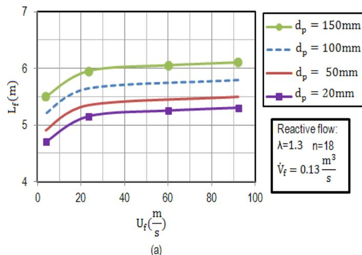
Fig. 6 Influence of fuel velocity (a) and lance diameter (b) on flame length
