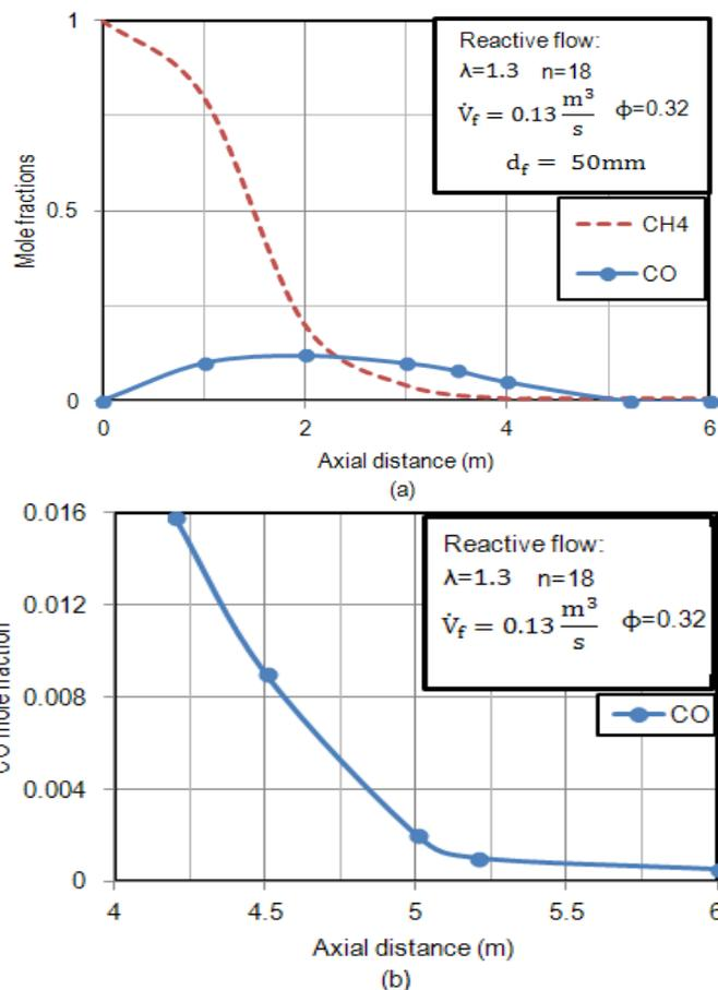
Fig. 5 (a) Axial CH<sub>4</sub> and CO profiles, (b) CO profile of H=4-6m
