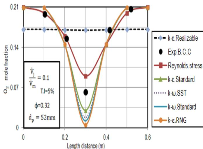
Fig. 3 Oxygen profile for different turbulence models and measured values (B.C.C. arrangement)
