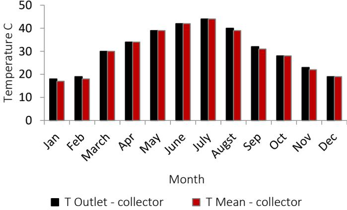
**Fig. 8** Mean and outlet monthly temperatures of solar collector of SWHS proposed
