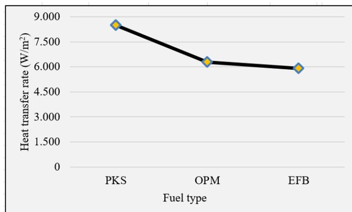
Fig. 8 Heat transfer rate (w/m) for different fuel
