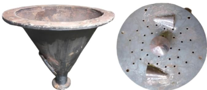
Fig. 2 Perforated plate modification for access air
