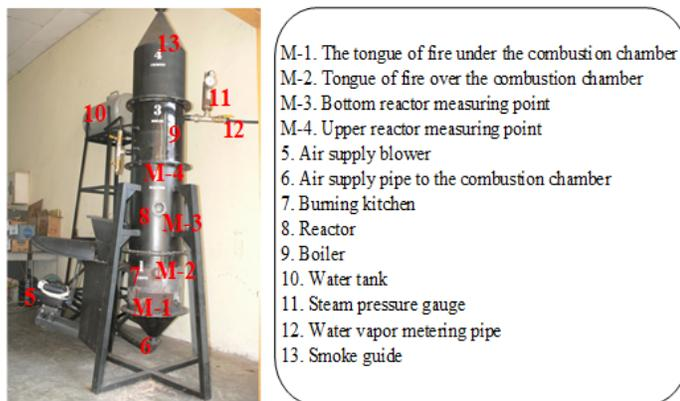
Fig. 1 Schematic Diagram for FBC
