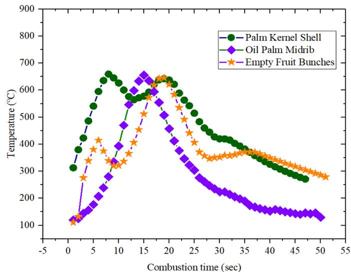
**Fig. 11** Profile temperature for different fuel time combustion in the M-IV
