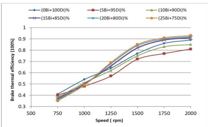
**Fig. 4** The effects of biodiesel rate on  $\eta_{bth}$  at different speeds.
