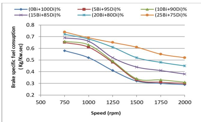
**Fig. 3** The effects of biodiesel rate on BSFC at different speeds.
