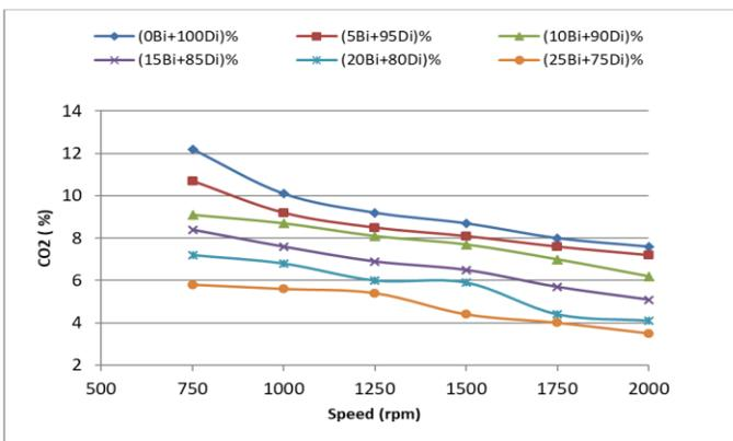
**Fig. 5** Effects of different biodiesel rates on CO<sub>2</sub> emissions at different speeds.
