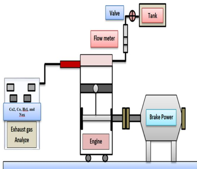
**Fig. 1** Experimental setup of the rig.
