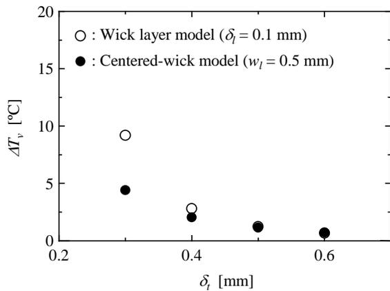
**Fig. 5** Vapor temperature differences with respect to the thickness of the heat pipe model ( $w_c = w_l = 1.5$  mm,  $l_c = 10$  mm).
