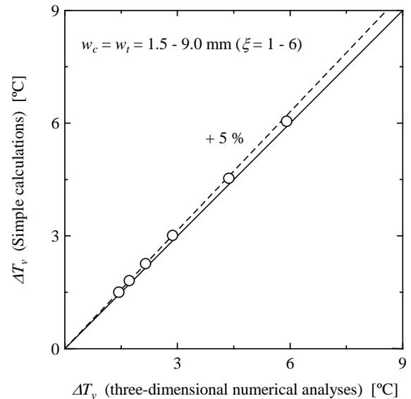
**Fig. 9** Comparison between the results of simple calculations and three-dimensional numerical analyses.
