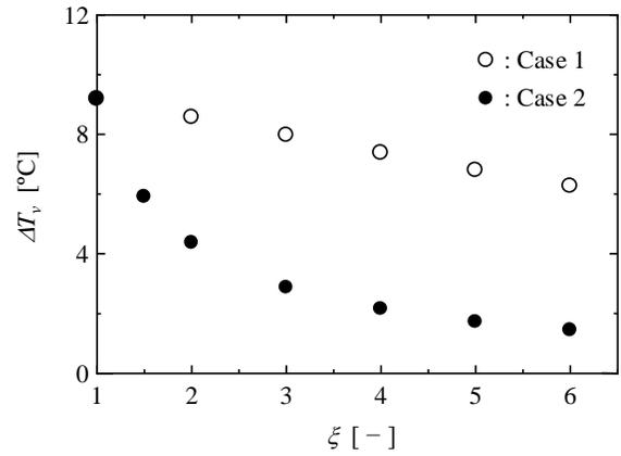
**Fig. 8** Reduction in the vapor temperature difference ( $\delta_l = 0.1$  mm,  $\delta_t = 0.3$  mm).
