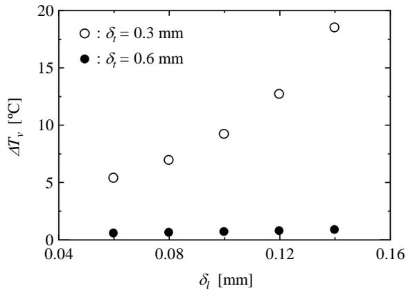
**Fig. 4** Vapor temperature differences with respect to the thickness of the liquid-wick region ( $w_c = w_l = 1.5$  mm,  $l_c = 10$  mm).
