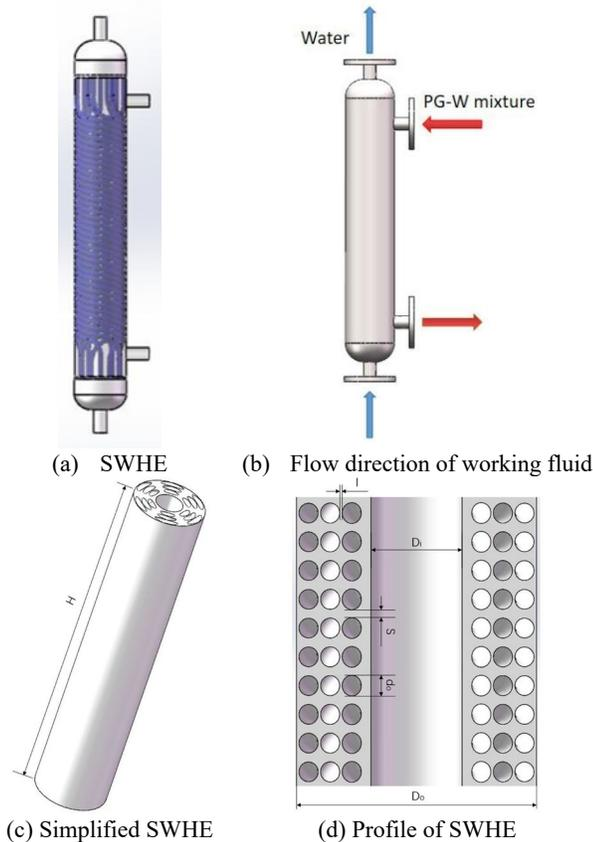
**Fig. 1** Physical model of SWHE
