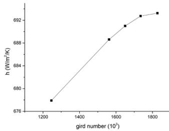
**Fig. 3** Heat transfer coefficient of different kind of grid
