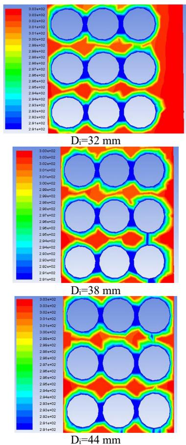
**Fig. 7** Temperature nephogram under different  $D_i$  (concentration is 30%, volume flow rate is  $0.6 \text{ m}^3/\text{h}$ )
