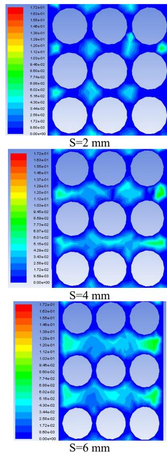
**Fig. 9** Flow nephogram under different  $S$  (concentration is 10%, volume flow rate is  $0.6 \text{ m}^3/\text{h}$ )
