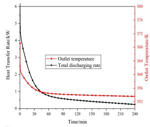
**Fig. 10** The evolution of the HTF outlet temperature and the total charging rates between the HTF and the PCMs during the discharging time.
