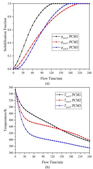
**Fig. 9** The evolution of: (a) volume-average solidification fractions, (b) mass-average temperatures for PCM1-PCM3 during the discharging process.
