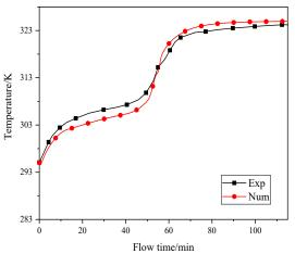
Fig. 3 Comparison of the predicted temperature variation with the present numerical model (Num.) and the experimental data (Exp.).
