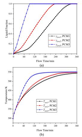
**Fig. 5** The evolution curves of PCMs during the charging process: (a) volume-average liquid fractions, (b) mass-average temperatures.
