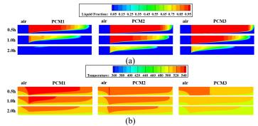
**Fig. 8** The contours of (a) liquid fraction and (b) temperature for PCM1, PCM2, and PCM3 during the discharging process.
