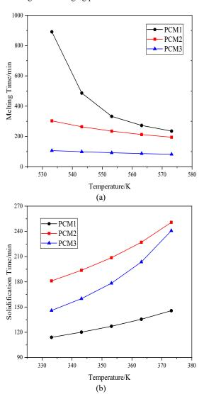
**Fig. 12** The changes of the melting time during the charging process (a) and the solidification time during the discharging process (b) with different HTF inlet temperatures.
