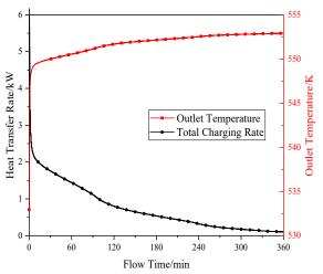
**Fig. 6** The evolution curves of the outlet HTF temperature and the total charging rate between the HTF and the PCMs with time.
