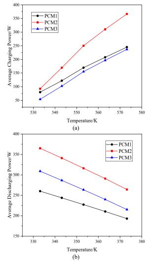
**Fig. 13** The change of the average charging and discharging powers as a function of the inlet HTF temperature.
