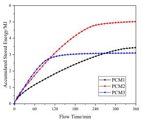
**Fig. 7** The evolution curves of the accumulated stored energy of the PCMs during the charging process.
