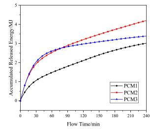
**Fig. 11** The evolution of the accumulated released energy of the PCMs during the discharging process.
