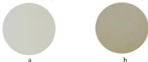
Fig. 6 The comparison diagram of water sample (a) Water sample in the pottery container for four days (b) Original water sample from a river
