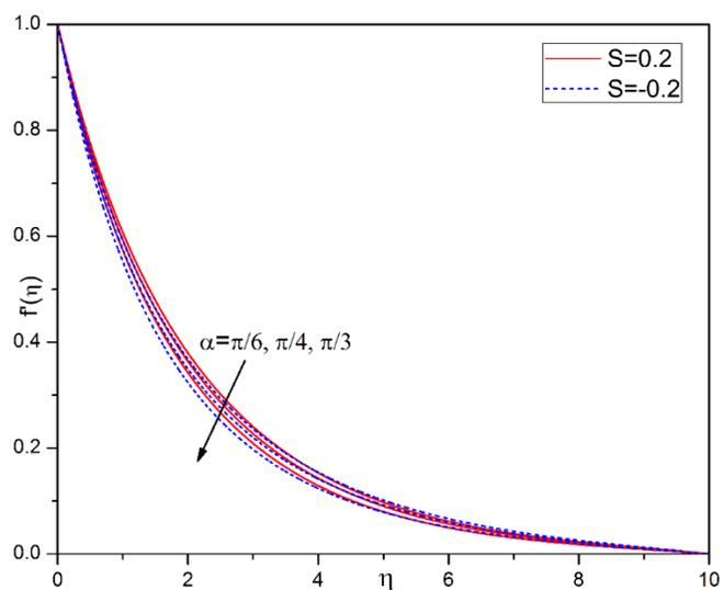
Fig. 3 Effects of  $\alpha$  on Velocity profiles
