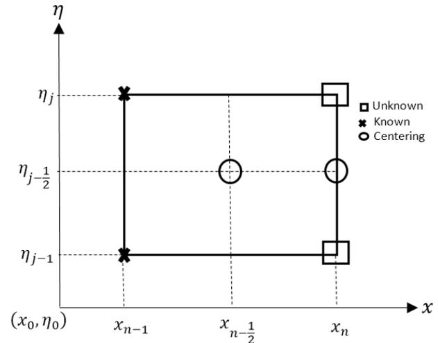
Fig. 2 Net rectangle for finite difference approximation
