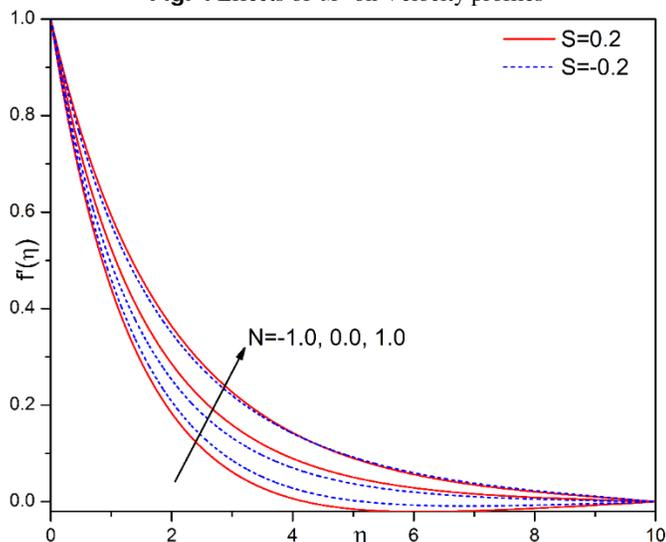
Fig. 5 Effects of  $N$  on Velocity profiles
