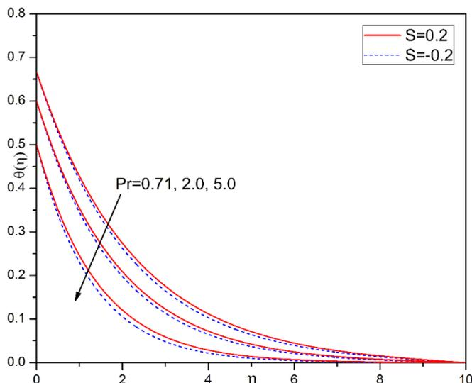
Fig. 10 Effects of  $Pr$  on Temperature profiles
