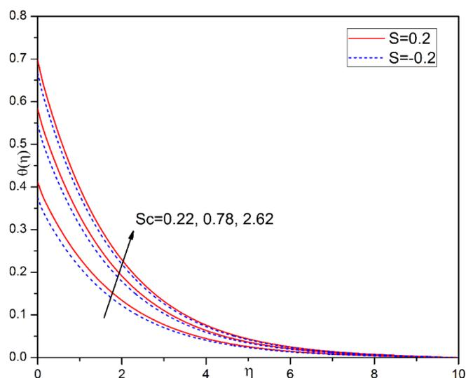
Fig. 12 Effects of  $Sc$  on Temperature profiles
