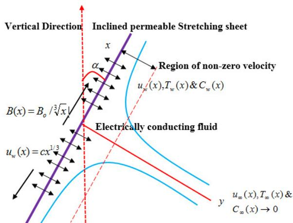
Fig. 1 Geometry and coordinate system for inclined stretching sheet
