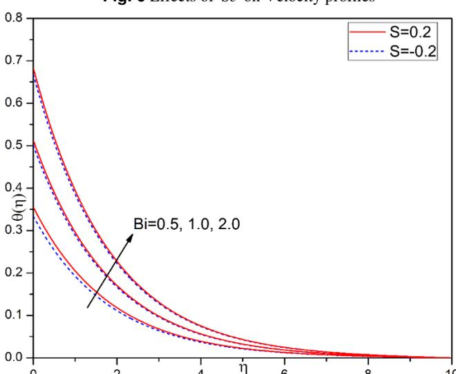
Fig. 7 Effects of  $Bi$  on temperature profiles
