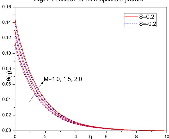
Fig. 8 Effects of  $M$  on Temperature profile
