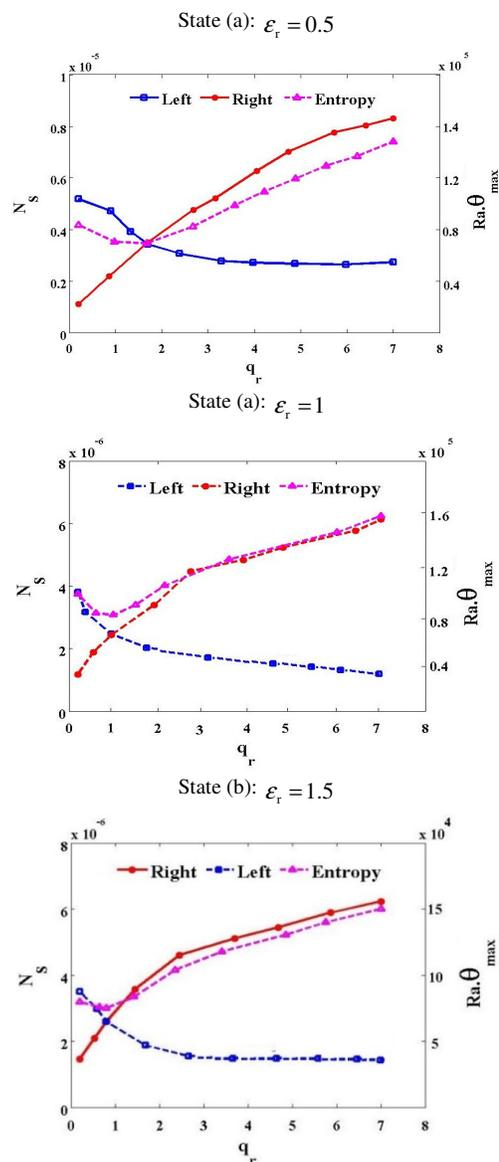
**Fig. 9** Variations in heater temperature and total entropy generation by changing power ratio of heaters
