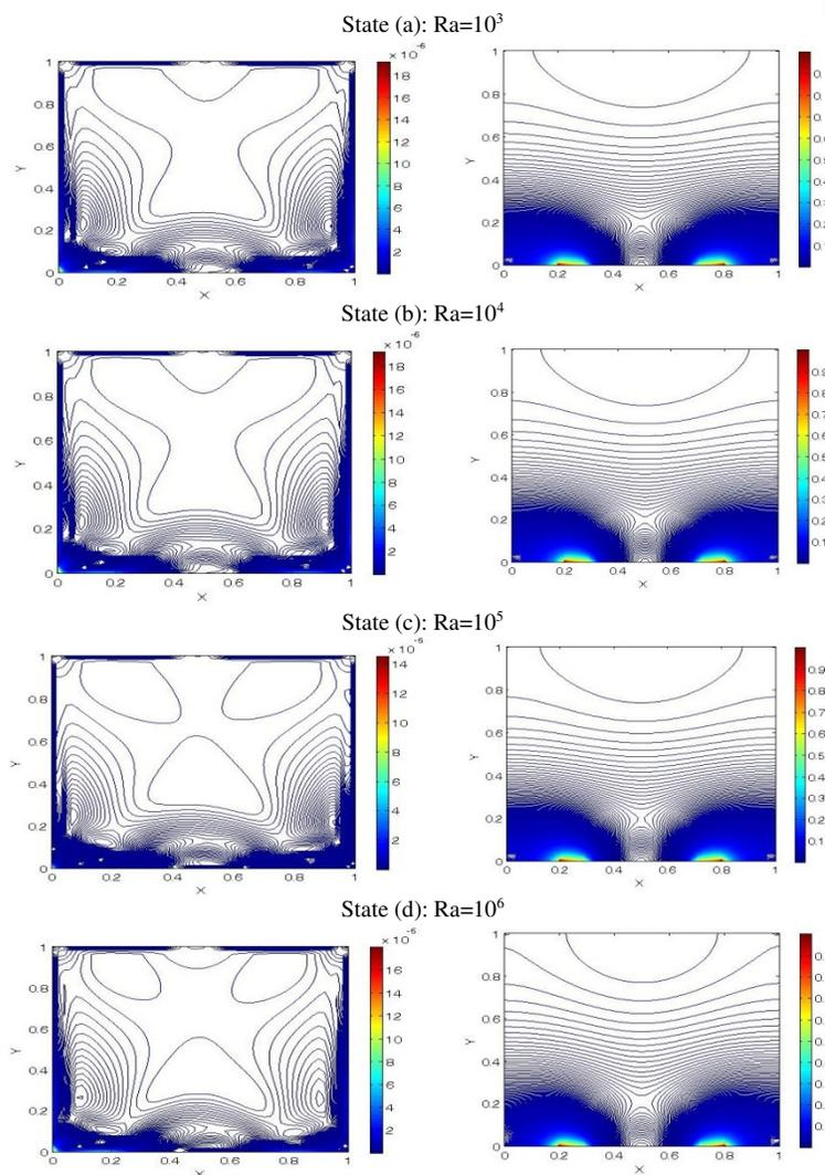
**Fig. 4** Variations in entropy generated by fluid friction (left column) and conductive heat transfer (right column) by changing the Rayleigh number
