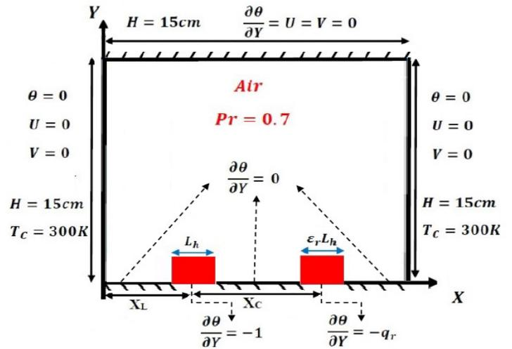
Fig. 1 Geometry of the problem with boundary conditions
