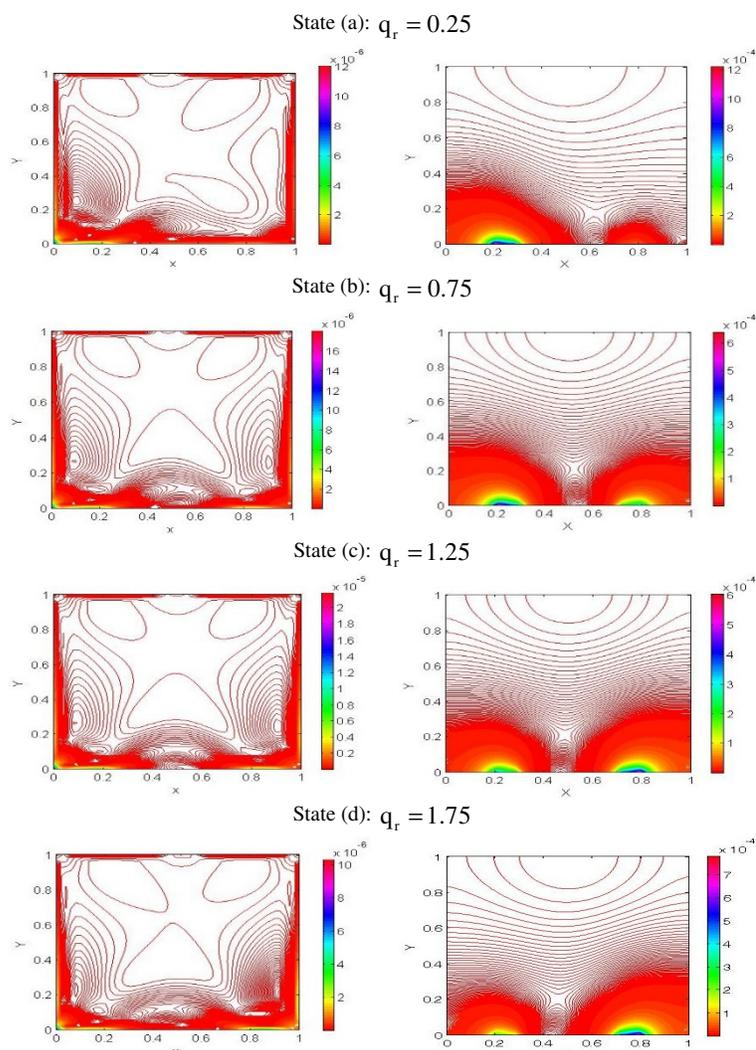
**Fig. 8** Variations in total entropy generation (right column) and entropy generation caused by fluid friction (left column) by changing power ratio of heaters
