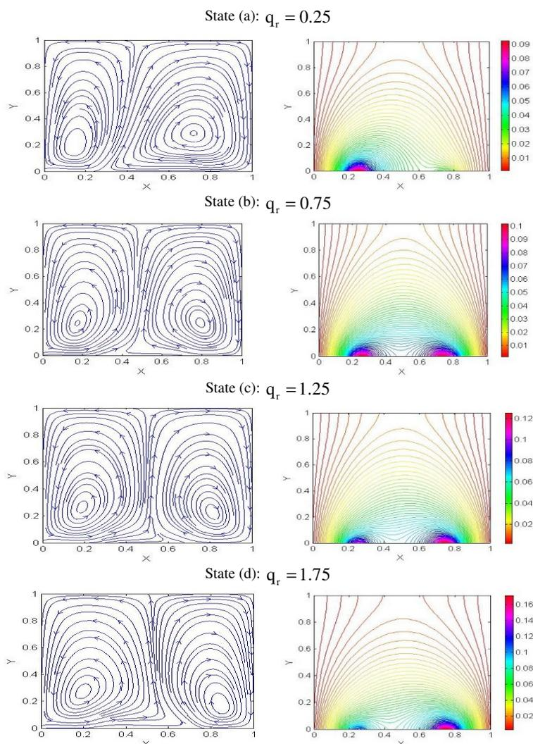
**Fig. 6** Variations in streamlines (left column) and isotherms (right column) by changing flux ratio of heaters
