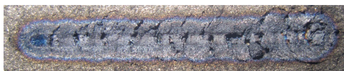
Fig. 7 Sintering result of titanium/nickel mixture (average power is 5.4 W, scanning speed is 0.1 mm/s, and repetition rate is 3000 Hz)
