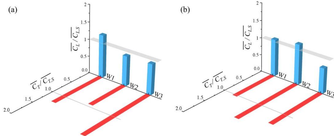
**Figure 4:** The ratio of the cycle-averaged lift and thrust coefficients to the single wing for each individual in (a) case A and (b) case B.
