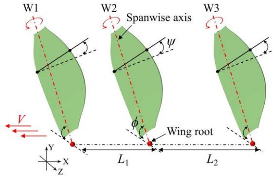
**Figure 1:** Schematic diagram of three flapping wings in tandem formation flight.
