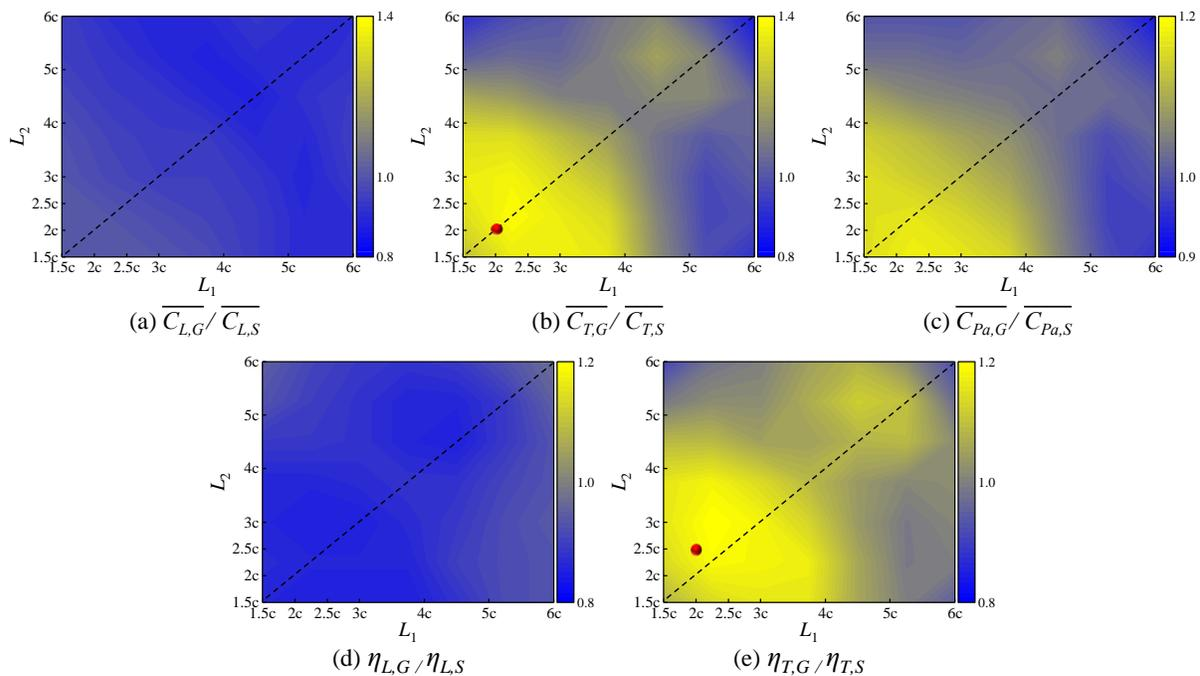
**Figure 3:** The ratio of the cycle-averaged lift (a), thrust (b), aerodynamic power (c), lift efficiency (d), and thrust efficiency coefficients (e) of the three flapping wings group to that of the single-wing for all tandem formation configurations. Subscripts “G” and “S” in the symbols represent the three-wing group and single wing, respectively.
