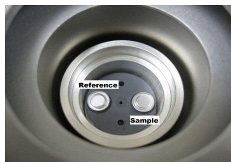
Fig. 3. Crucible Placed on the Heat Flux Sensor
