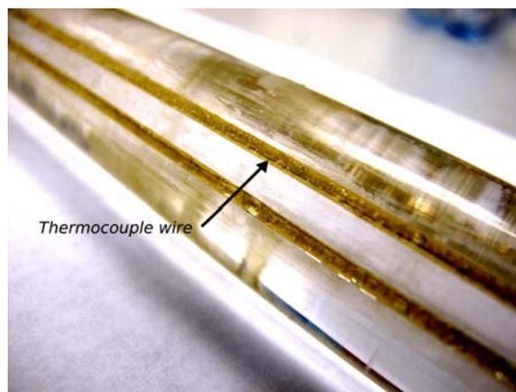
**Figure 5** Close up of an acrylic preform with embedded thermocouple (wire).
