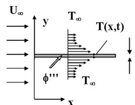
**Fig. 1** Thin plate with uniform heat generation and convectively cooled from both surfaces.
