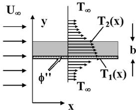
**Fig. 3** A plate with uniform heat generation  $\phi''$  at lower surface and convection cooling at both surfaces.
