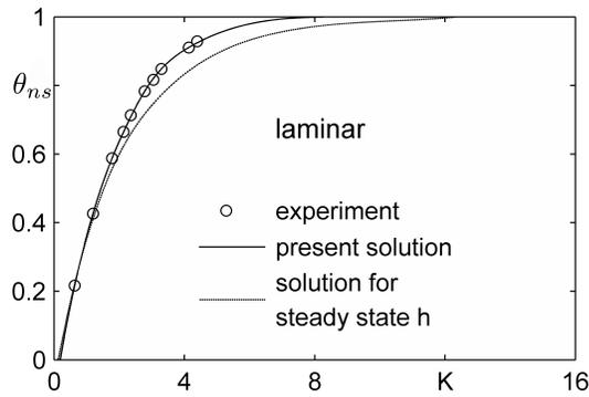
**Fig. 4** Thin plate transient temperature and comparison to measurements. Laminar flow.
