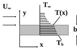
**Fig. 2** Plate with uniform temperature  $T_b$  at lower surface and convectively cooled at upper surface (Luikov problem).
