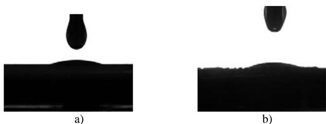
Fig. 7 HFE 7200 droplet on a) bare chip b) 4 $\mu$ m nanowire surface
