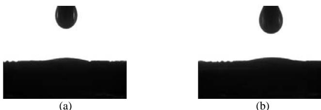
Fig. 8 Droplet of 10 vol% mixture of a) HFE 7200 – Ethoxybutane b) HFE 7200 – Methanol, on 4 $\mu$ m nanowire surface
