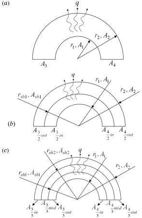
Fig. 1. Top view of two long concentric semi-cylinders: (a) without radiation shield, (b) with one radiation shield, and (c) with two radiation shields
