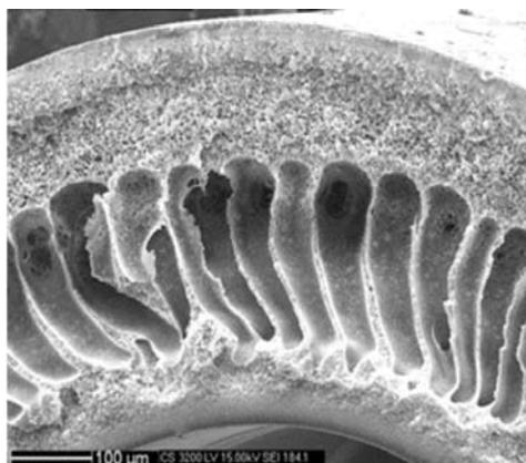
c. Magnified view of top layer of cross section
