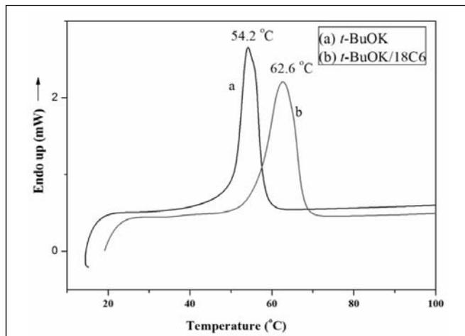
Fig. 3. DSC curves of PCL (Table 1, entries 1 and 4).
