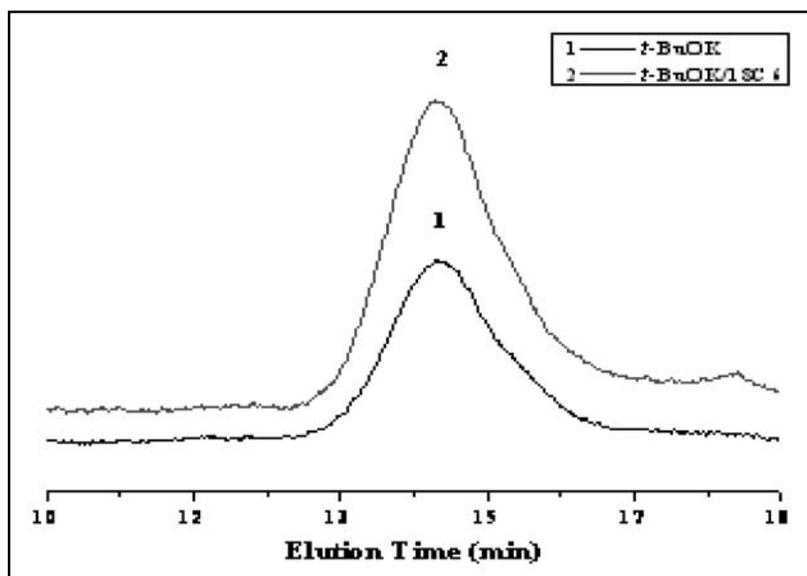
Fig. 2. Typical GPC curves of PCL (Table 1, entries 1 and 4).
