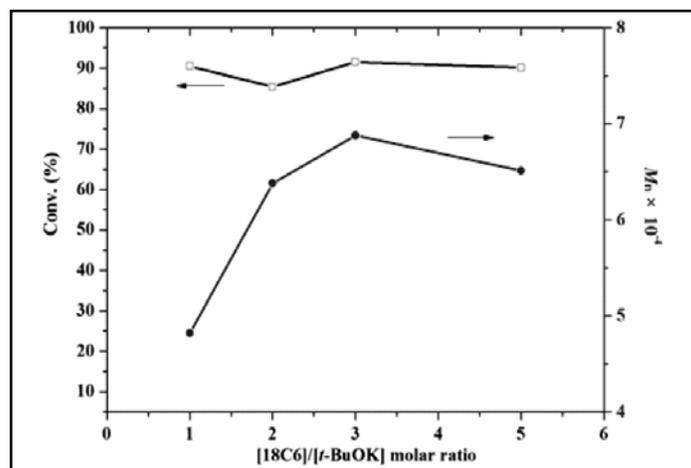
Fig. 1. Effects of molar ratio 18-crown-6/*t*-BuOK on  $\epsilon$ -CL polymerization
