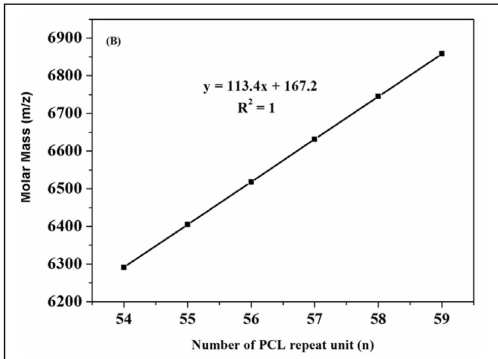
Fig. 7. MALDI-ToF MS spectrum of the obtained PCL sample (Table 2, entry 6) in the positive linear mode (A). Detail including experimentally observed mass; (B) the plot of the molar mass ( $m/z$ ) versus the number of monomer repeat units ( $n$ ).
