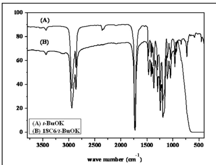
Fig. 5. FTIR spectra of PCL: (A) PCL obtained by *t*-BuOK/18C6 initiator system (Table 1, entry 4) and (B) PCL obtained by *t*-BuOK initiator system (Table 1, entry 1).
