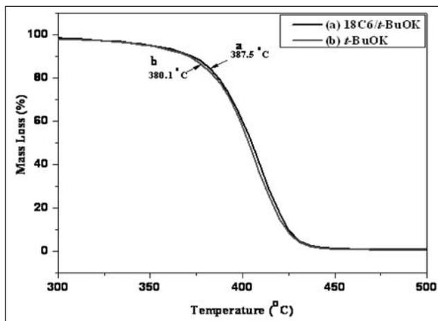
Fig. 4. TGA curves obtained at 10 °C min<sup>-1</sup> under a nitrogen atmosphere: (a) PCL sample initiated by *t*-BuOK/18C6 (Table 1, entry 4); (b) PCL sample initiated by *t*-BuOK (Table 1, entry 1).
