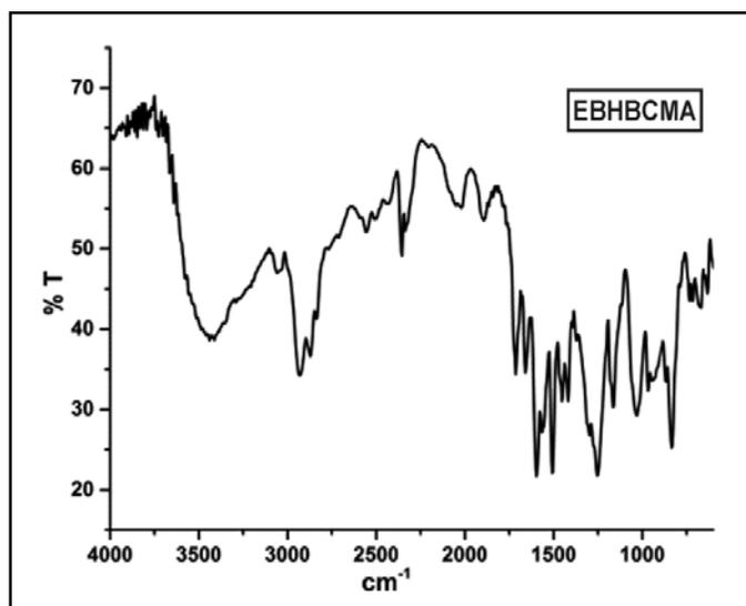
Fig. 2. FT-IR spectrum of EMBHBCMA.
