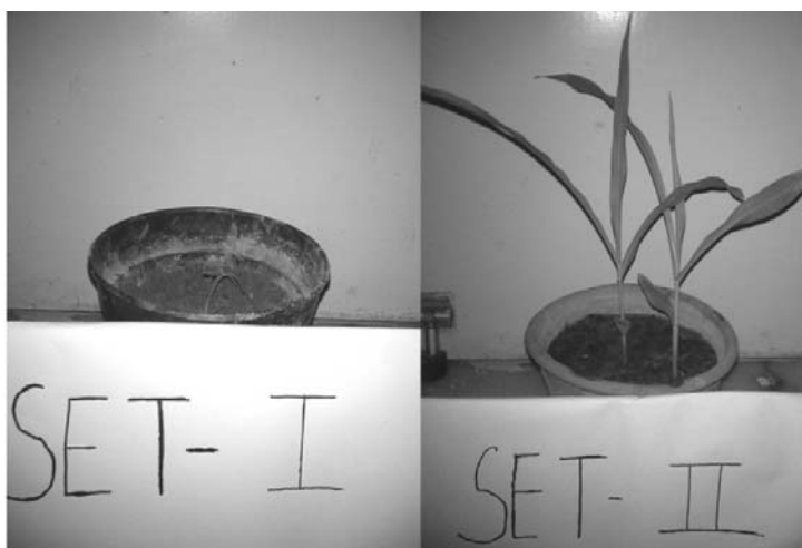
Fig. 7. Growth of corn, SAHs S_3 act as a soil conditioner for set-I ; 0.0%SAH and set-II 0.4 % SAH(based on soil weight)
