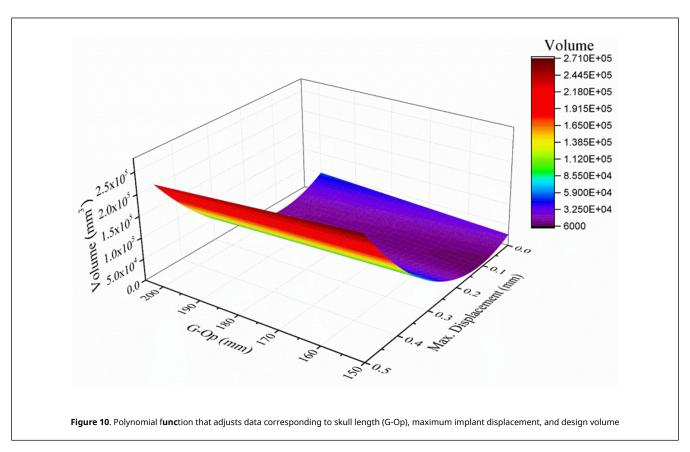
Finally, the optimal designs for each percentile were found using the solver tool, which minimizes the amount of material (Ti6Al4V) while maintaining a maximum displacement of 0.1 mm. The optimal designs are shown in  $\underline{\text{Table 8}}$  and were obtained with the minimum volume by Eq.(7) as the objective, using the maximum displacement of Eq.(8) as a restriction (minor or equal to 0.1 mm). The maximum displacement of these designs was validated using MEF and shown in Table 8.
