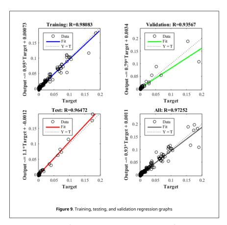
final volume of the implant, obtaining an  $R^2$  of 0.97. <u>Table 7</u> shows an adjusted  $R^2$  of 97.31%, indicating that the model can estimate the volume using the design variables as predictors.
