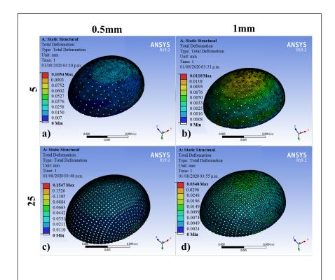
**Figure 6.** Results of the cranial implant simulations with an applied force of 2000N corresponding to design number. (a) 3 (percentile 25 with a thickness of 0.5 mm). (b) 4 (percentile 25 with a thickness of 1 mm). (c) 13 (percentile 50 with a thickness of 0.5 mm). (d) 14 (percentile 50 with a thickness of 1 mm)
