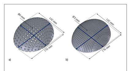
**Figure 3.** 3D design of the skull implant with 0.5 mm of a thickness corresponding to the dimensions of the 5<sup>th</sup> percentile using (a) 10° with 6 mm of diameter and (b) 5° of separation with 3 mm of diameter
