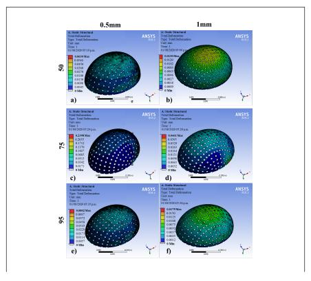
**Figure 7**. Results of the cranial implant simulations with an applied force of 2000N corresponding to design number. (a) 31 (percentile 50 with a thickness of 0.5 mm). (b) 32 (percentile 50 with a thickness of 1 mm). (c) 47 (percentile 75 with a thickness of 0.5 mm). (d) 48 (percentile 75 with a thickness of 1 mm).
