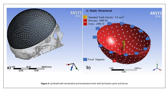
The mechanical properties of implants were all treated as isotropic, homogeneous, and linear elastic. Therefore, the safety factor is high in all the proposed designs, and large deformations are not considered since the element is expected to deflect (maximum displacement of 0.1 mm), but without exceeding the yield point, the element does not reach the plastic failure.
